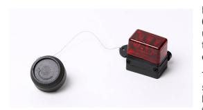
Phoenix<sup>™</sup> Jr. Intruder Beacon System (NSN: 5855-01-539-0639) is a trip wire activated infrared beacon used in conjunction with night vision equipment to detect and signal night movement along trails, roads and entry points.
