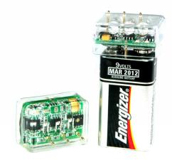
Phoenix<sup>™</sup> 2.5 (NSN:5855-01-451-9877) is a programmable infrared signaling beacon designed for during low light operations.
