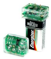
**Pegasus™ 10** is a flashing infrared signaling beacon designed for use during low light operations. Engineered as an enhancement of the Phoenix Jr. (Firefly) (NSN: 5855-01 -438-4588) infrared beacon, the Pegasus 10 provides the same fixed flash pattern, but with the ability to adjust the beacons signal brightness.
