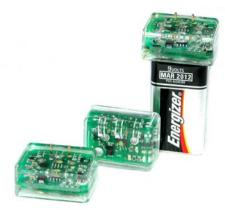
**Pegasus™ 12** is an infrared signaling beacon designed for use during low light operations. Engineered as an enhancement of the Phoenix series of infrared beacons, the Pegasus beacon series incorporates several encoding options within each Pegasus beacon.
