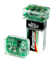
**Velux™** 1 is a programmable Short Wave Infrared (SWIR) signaling beacon designed for use during low light operations. Engineered as a beacon platform with the ability to broadcast 950nm to 1550nm, the Velux beacon series includes several encoding options.
